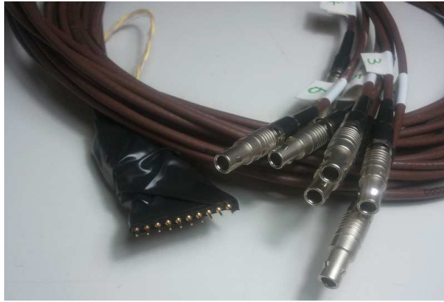
Figure 4.36: The custom LEMO cables used to connect the SiPM output signal to the MAROC input pins.
