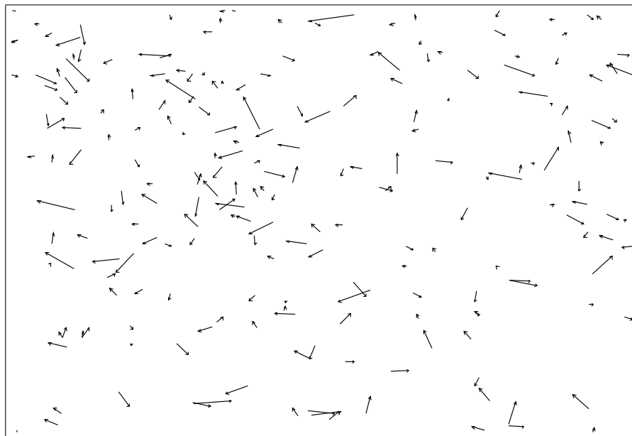
Figure 4.2: Typical distortion map of an emulsion. The arrows represent the difference between the micro-track and the base-track angle. This particular emulsion comes from a 2004 CERN test-beam Brick
