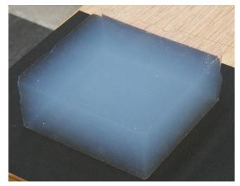
Transparent over a wide range: optical properties dominated by Rayleigh scattering: Transmittance T, clarity factor C, surface scattering factor A, thickness t, wavelength  $\lambda$
