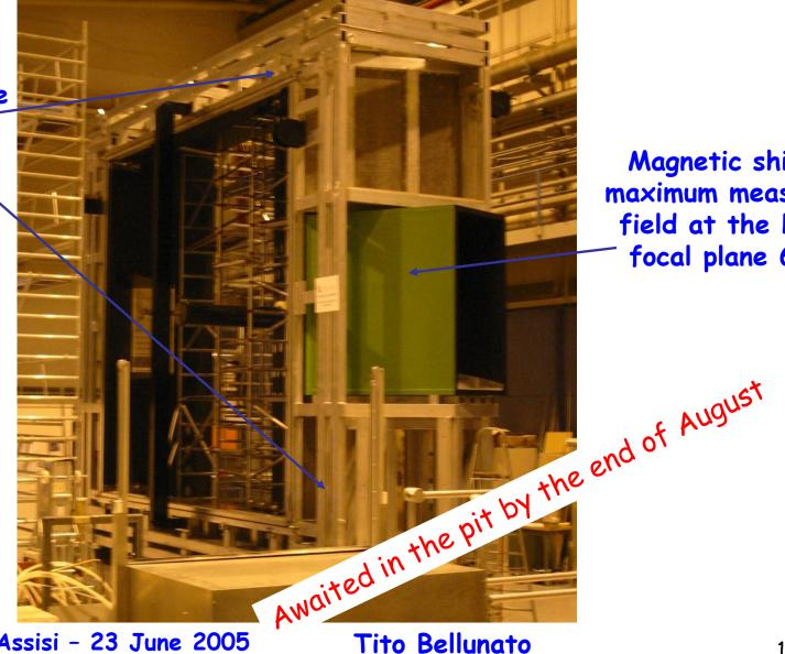
Magnetic shield maximum measured field at the HPD focal plane 6 G
