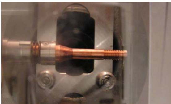
Figure 3. Modified photocathode stem with grooves for multipacting suppression.
