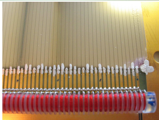
Figure 3.5: In the top picture the PPAC frame is shown before the installation of the electrodes. In the middle, PPAC appearance where the stripped cathode, the delay line on one side and some preamplifiers are shown. In the bottom, a delay line detail showing how each cathode strip is soldered to a delay line rod.
