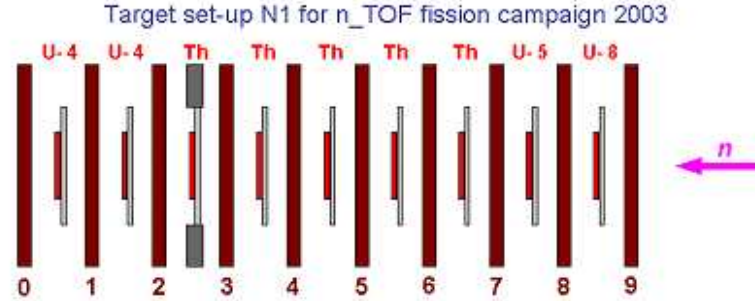
Figure 3.7: Schematic view of the ^{234}\text{U} and ^{232}\text{Th} setup used during the 2003 campaign. The detectors are labelled by their numeration in the arrangement; the same convention is used with the targets.
