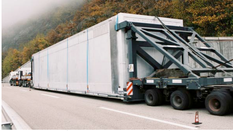
Figure 15: Picture taken during the transportation of a T600 half-module to LNGS. One of the two trolleys, attached to the aluminium vessels rear side, is well visible.
