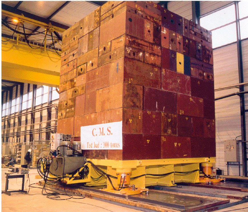
Figure 33. 1000 t test load being moved on a system of 4 high pressure air pads.
