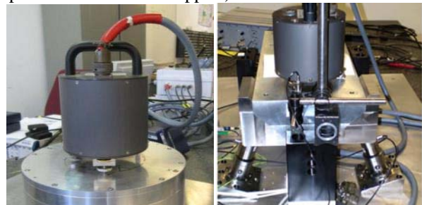
Figure 1: Two demonstration benches: left: single d.o.f. system (membrane), right: two d.o.f. system (tripod) with 100 kg dummy magnet mass.
