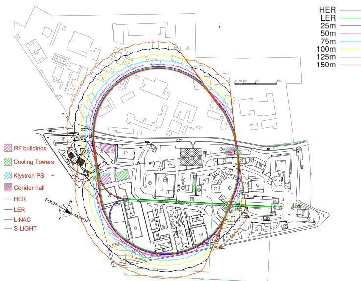
Figure 8: All possible bend magnet photon beam line location with different contour lines showing the distance to the source point.
