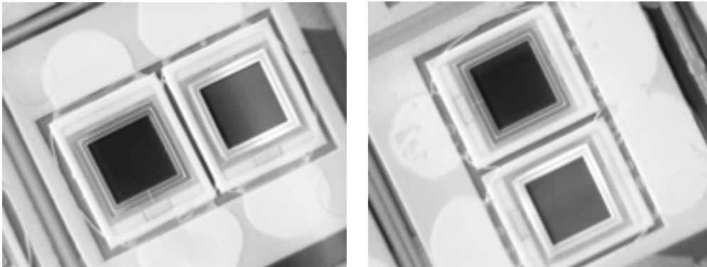
Figure 6.16: Pictures showing two gluings performed for Module 0' using RTV 3145.
