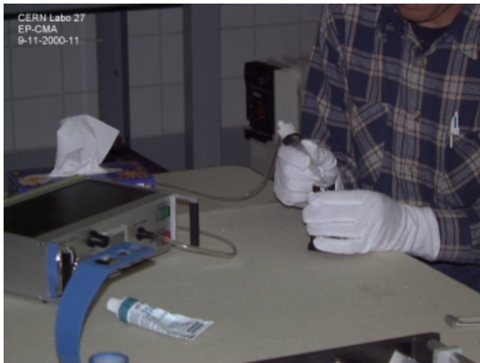
(b) Operator placing glue drops on a capsule
