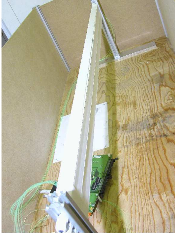
Figure 3.16: A photo of the five triangular long bars connected to the MAPMT + FEB prototype: each bar is 1.1 m long and is readout by two 0.8 mm diameter WLS fibers connected on both sides to the 64 channel MAPMT.
