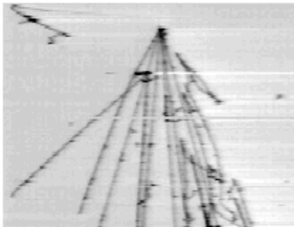
Figure 13 - An example of recorded neutrino interaction in the 50-litre LAr-TPC located at the CERN neutrino beam in 1997. The neutrino comes from the top of the picture. The horizontal axis is the time axis (drift direction) and vertically is the wire number. The visible area corresponds to 475 \times 325 \text{ mm}^2 .
