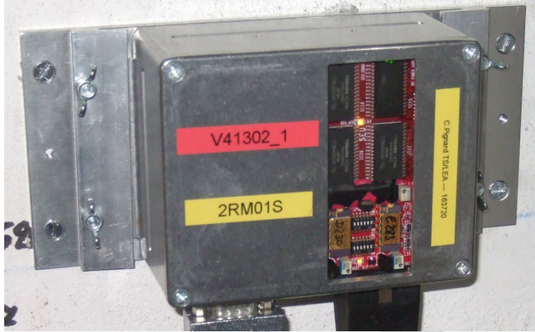
Figure 1: RadMon installed in the LHC. The 4 Toshiba SRAM memories can be seen at the top of the open window of the RadMon housing.
