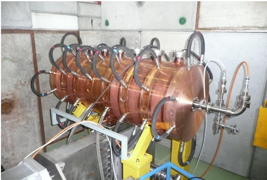
The PIMS prototype cavity shown at the 3 MeV Test Stand at CERN inside the bunker where it was tested with RF power.
