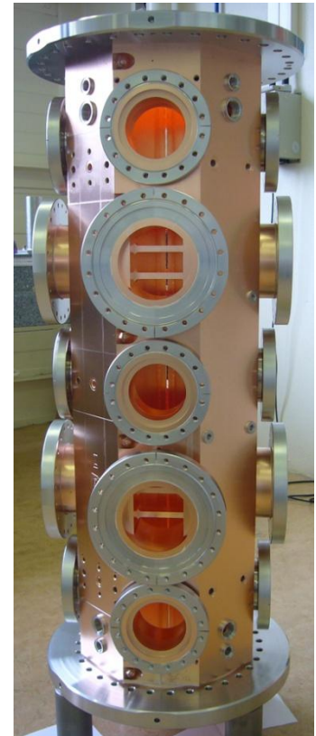
The first module of Linac4 RFQ after the second brazing step.
