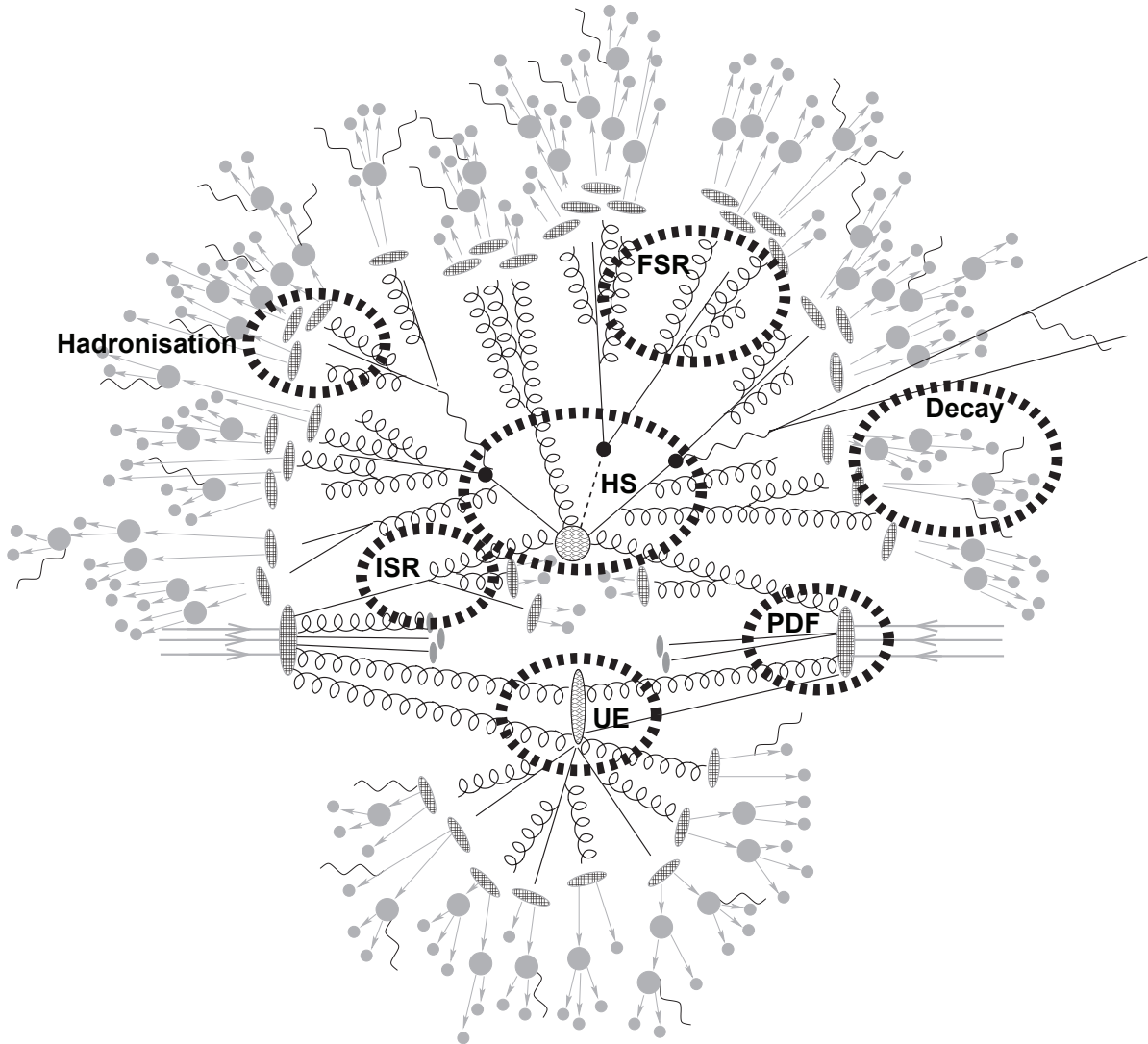
Figure 1.9: Schematic view of the production of t\bar{t}H + X in a pp collision. Shown in the ellipses are the various stages that need to be handled by simulation programs: the hard scatter (HS) which depends on the parton density function (PDF), initial and final state radiation (ISR and FSR), the hadronization and decay of particles and the underlying event (UE). Figure taken from [32,65].
