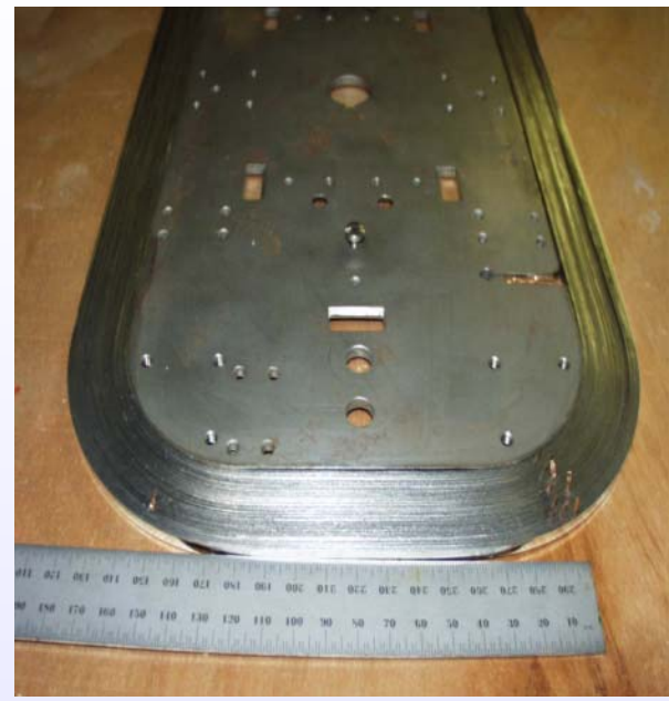
Cu thickness: SuperPower ~ 0.045 mm; ASC ~ 0.1 mm (width = 4 mm)
