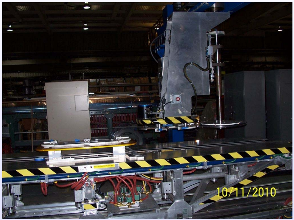
R&D coil ready to be wound with the 12 mm 2G tape
