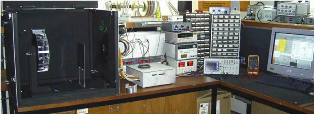
Figure 3.2: Early setup of a PDTF station at Edinburgh. It is largely unchanged even today. From left to right: darkbox where HPD is mounted, HV supply and electronics, MB & FB board for interfacing with the readout chip, other power supplies and picoammeter, all controlled by the PC through the JTAG controller. The oscilloscope checks the blackout conditions using a photomultiplier inside the darkbox.
