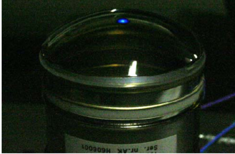
Figure 4.6: Light from a glowing HPD, visually observed in a dark room. The image is superimposed with a photograph of an HPD with external lighting to show the location of the light source. The image has been colour edited for clarity. This figure comes from [31].
