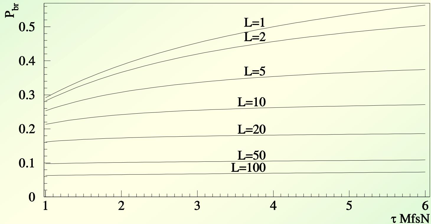
Probability of A2pi breakup in Ni targets consisting of layers with 1 mm gaps and total thickness of 100 mkm as a function of lifetime.
