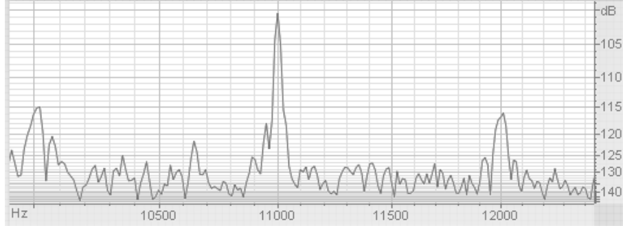
Figure 14: Spectrum during normal operation containing no higher losses. Only background noise from the environment is picked up with the microphone.
