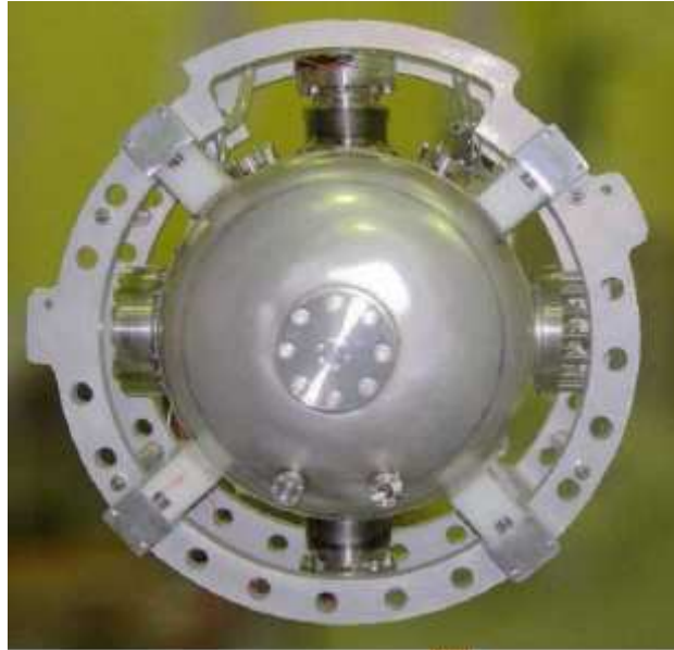
Fig. 2 Spoke cavity inside its cradle, blocked by Teflon pads.
