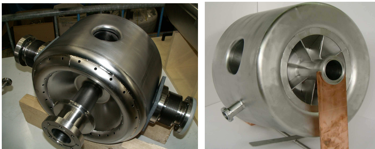
Fig. 3: Picture of the two single spoke superconducting cavities: \beta 0.15 (left), \beta 0.35 (right)
