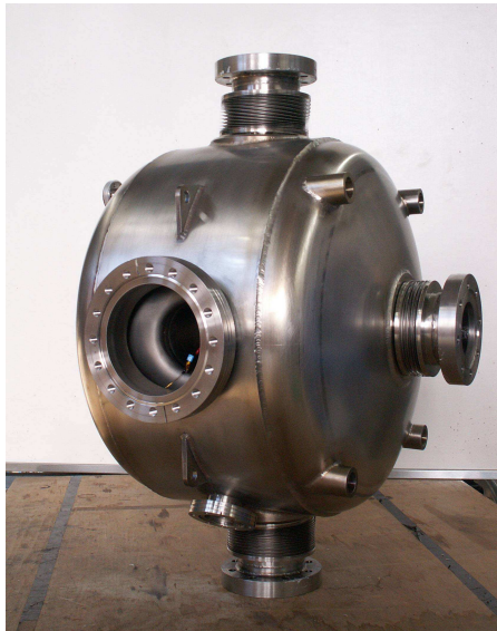
Figure 4:: Low beta spoke cavities after welding of the helium tank
