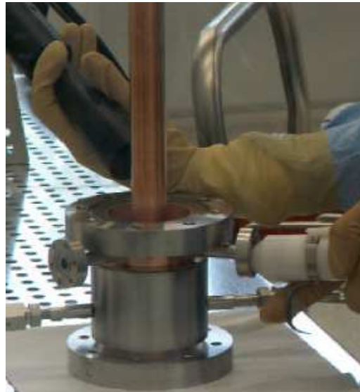
Figure 13a: Evaluation of the Power coupler cleaning procedure efficiency by performing a particle counting
