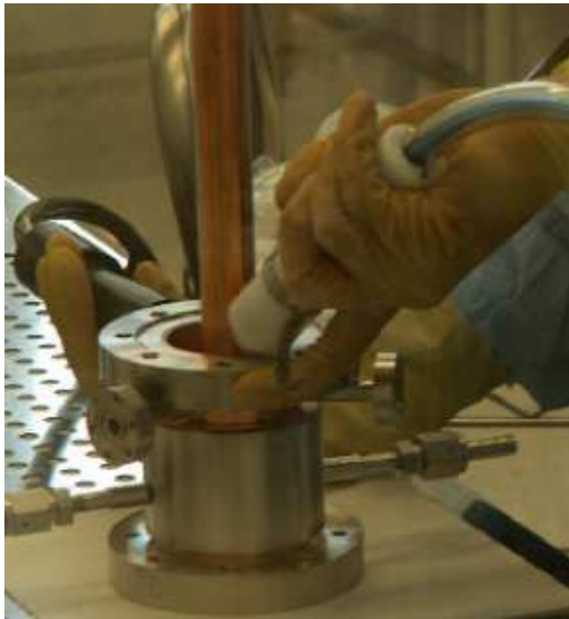
Figure 13a: Evaluation of the Power coupler cleaning procedure efficiency by performing a particle counting
