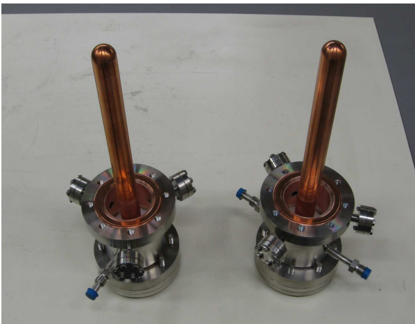
Figure 13b: The two power coupler prototypes (left) and the conditioning cavity assembly in the clean room
