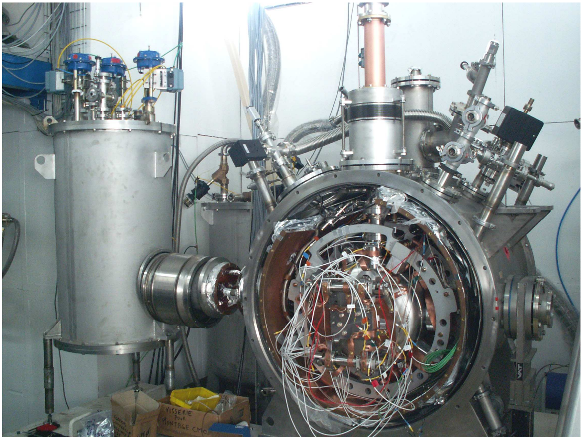
Fig. 8: Spoke Cryomodule and its cold box just before the cryogenic test.
