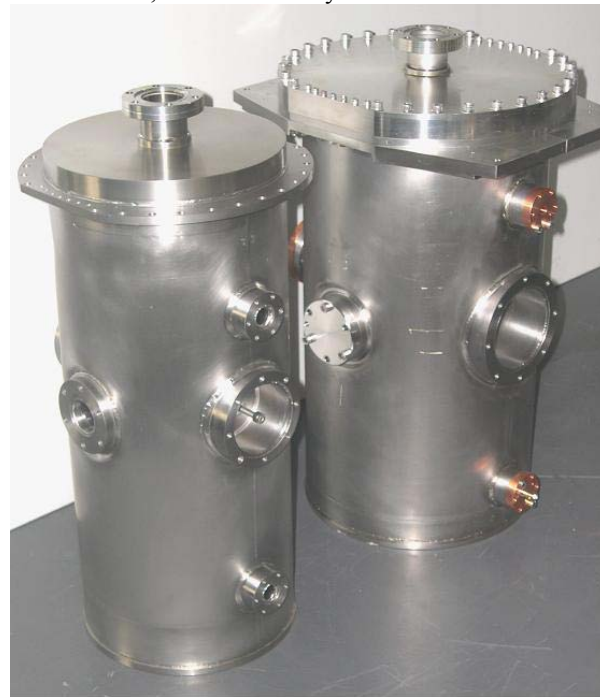
Figure 1: The INFN-LNL low- \beta (left) and medium- \beta 352 MHz superconducting Half-Wave-Resonators.
