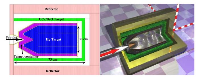
Figure 1. Schematic and artistic views of the baseline configuration, where several components of the Multi-MW target station have been integrated.
