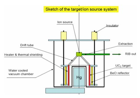
Figure 3. Integration sketch of different components of the Multi MW target [5], based on the baseline configuration.
