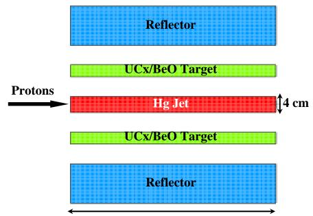
**40 cm Figure 2.** Schematic view of the Hg-jet option, where several elements of the facility have been included, as reported in [8].
