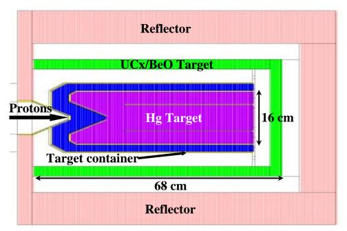
Figure 4. Schematic view of the scaled-down baseline configuration, showing different elements of the assembly.
