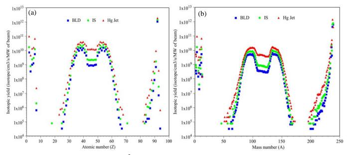
**Figure iii.** Fission yields (isotopes/cm<sup>3</sup>/s/MW of beam) in the three different configurations as a function of the atomic number Z (a), and the mass number A (b).
