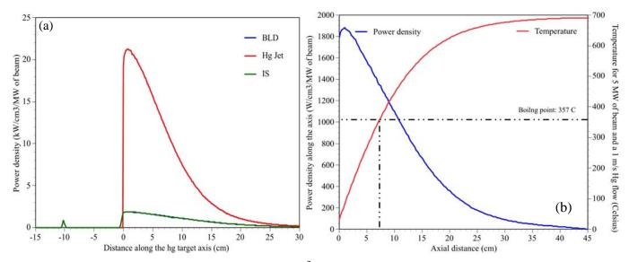
**Figure ii.** Power density distribution  $(kW/cm^3/MW \text{ of beam})$  for the three Multi-MW target configurations studied (a), and power density distribution and temperature increase along the beam axis for the baseline configuration and its scaled-down version.
