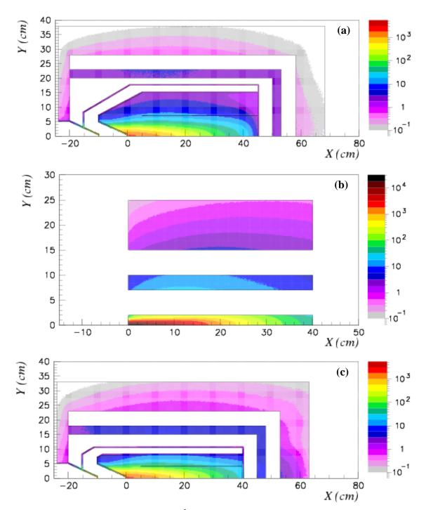
Figure 8. Power density distribution  $(W/cm^3/MW \text{ of beam})$  in (a) baseline configuration, (b) Hg-jet option and (c) scaled-down version.
