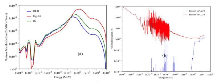
**Figure i.** Neutron energy spectra (dn/dlnE/cm<sup>2</sup>/s/MW of beam) for the three different Multi-MW target configuration (a), and fission cross-section comparison for  $^{235}$ U and  $^{238}$ U (b).
