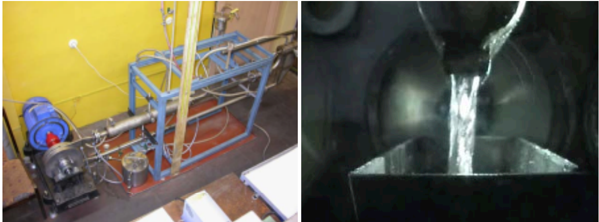
Figure 10. View of the liquid metal experimental loop (a), including the magnetic pump (to the left, in blue). Front view of the liquid metal transverse film (b).
