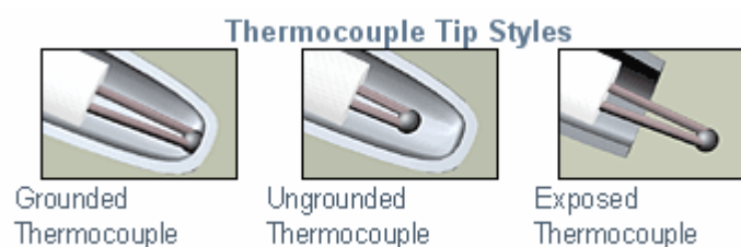
Figure 42: Thermocouples tip styles [http://www.omega.com/prodinfo/thermocouplesensor.html]
