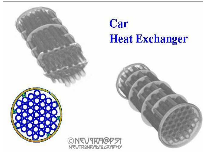
Figure 12: Neutron radiography (Car heat exchanger)
