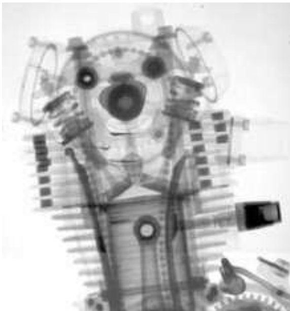
Figure 11: Neutron radiography (engine)
