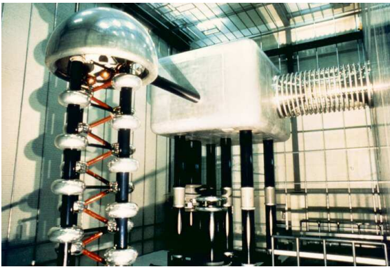
Figure 3: Proton source and Cockcroft-Walton accelerator at PSI Figure 4: C-W cascade generator [Wille]
