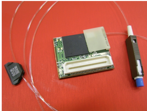
Figure 4.15.: The gigabit optical hybrid chip with the fibre pigtail and the connector.
