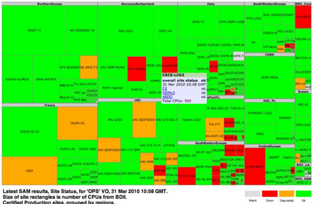
Figure 5.2: GridMap shows a visualization of the status of WLCG. The number of CPUs and status of sites are represented by rectangles of different sizes and colors respectively. The Swiss Tier-2 (CSCS-LCG2) is shown in the middle of the graph. The pop-up dialog box shows the overall status of the Swiss Tier-2 site. [http://gridmap.cern.ch]
