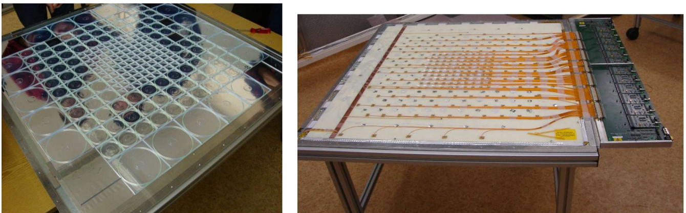
Figure 27. Scintillator tiles layer (left), assembled module with front end electronics (right).
