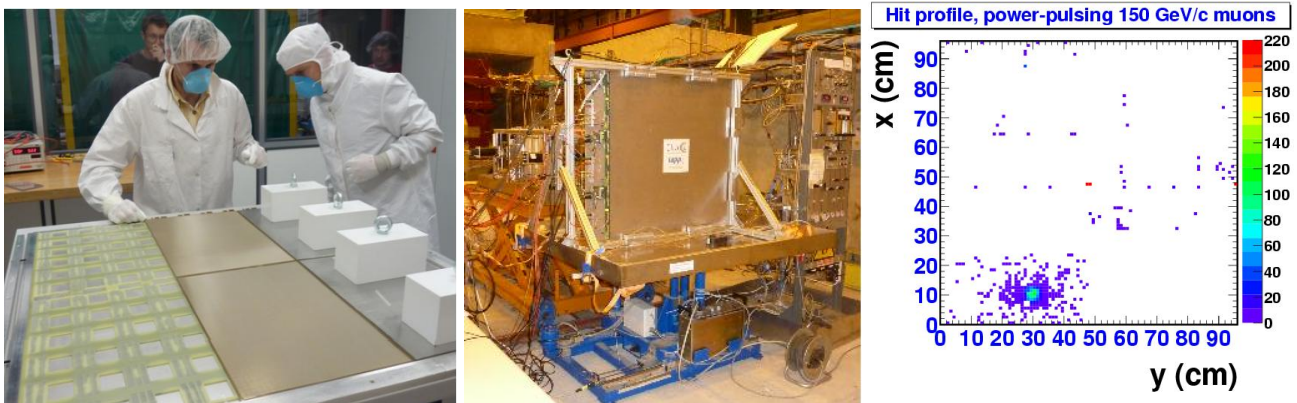
Figure 44. From left to right: assembly of the 1 \text{ m}^2 MICROMEAS prototype, test setup in CERN/SPS/H4 line in June 2010 and recorded muon beam profile.
