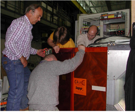
Figure 45. From left to right: Insertion of the m^2 MICROMEAS prototype inside the last slot of the AHCAL-tungsten structure in CERN/PS/T9 line in November 2010. Number of hits measured at various beam energies and projection of the hits recorded at -10 GeV/c along the horizontal direction showing the contributions from beam muons, electromagnetic shower core and hadronic halo.
