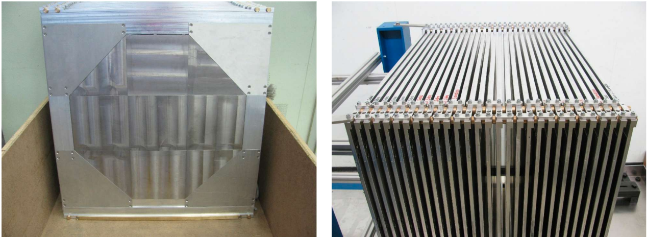
Figure 26. View of W-HCAL absorber plates (left) and stack during assembly(right).
