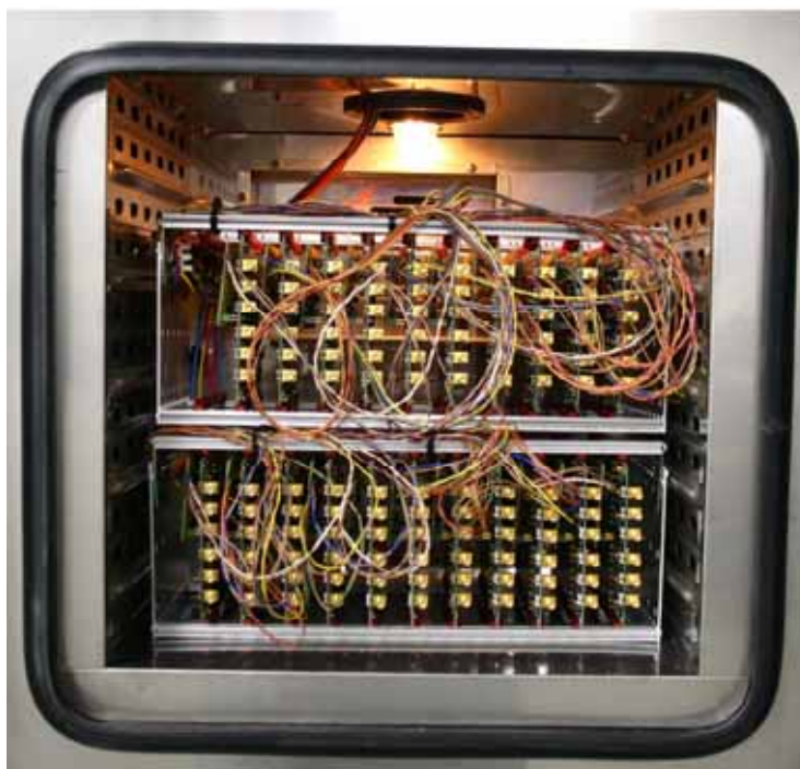
Figure 80 – Up to 22 FEBs were placed in a climate chamber for burn-in under electric power.
