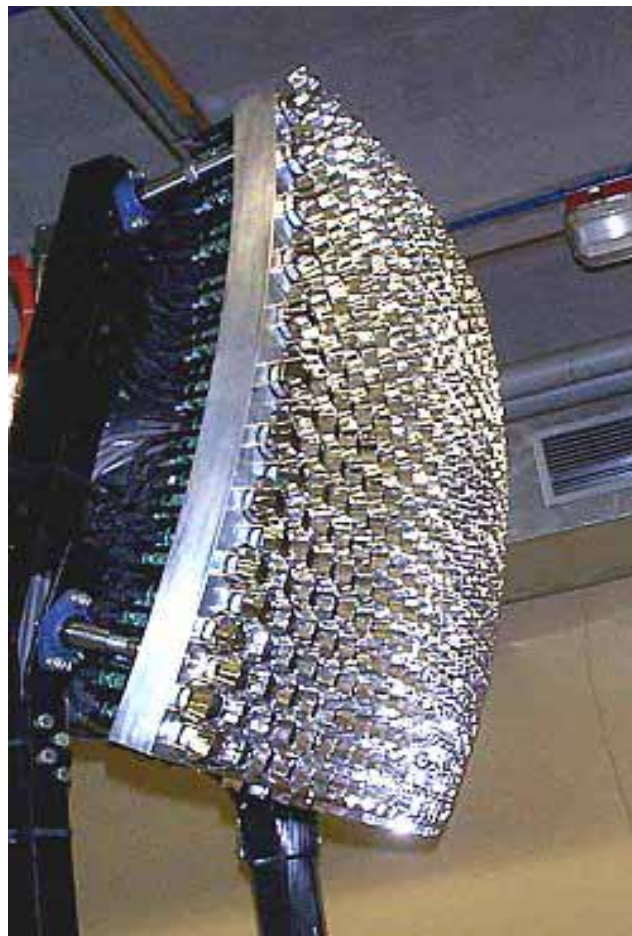
Figure 9 – A view to a Fluorescence Detector camera with 440 hexagonal PMT.
