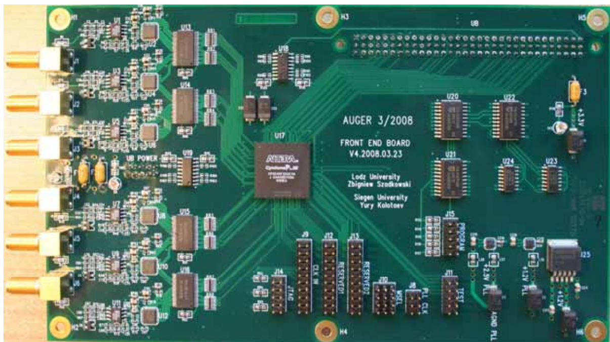
Figure 98 – The prototype Front End Board with the single FPGA Cyclone III [58].
