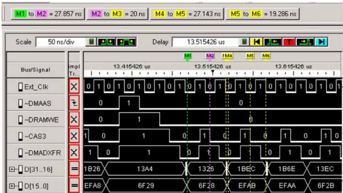
Figure 76 – The logic analyzer view of the slow 1WS DMA transfer for Cyclone™ (an short interruption for dynamic memory refreshment). PLL parameters are optimized for the fast channel as more critical. For the slow channel ~CAS3 occurs not in the middle of the stable data, however the hold time on the level 20 ns is still much higher than a required 10 ns.
