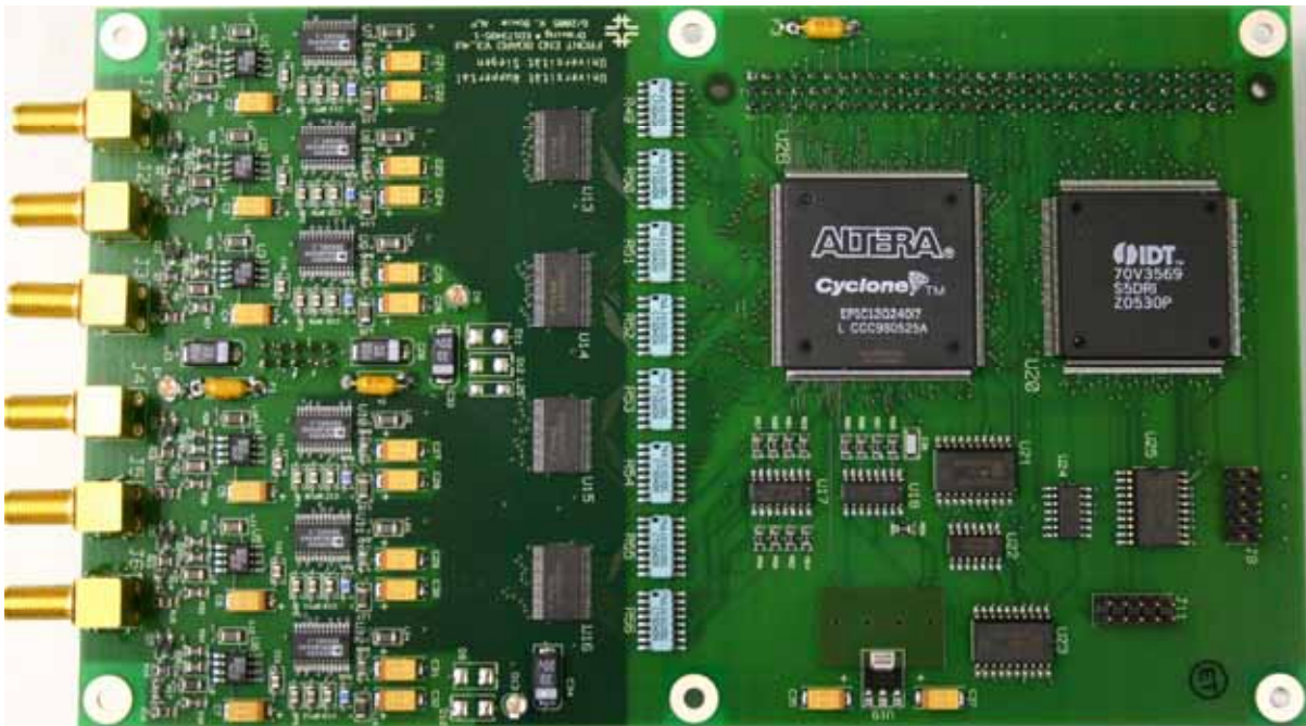
Figure 86 – Cyclone prototype board.
