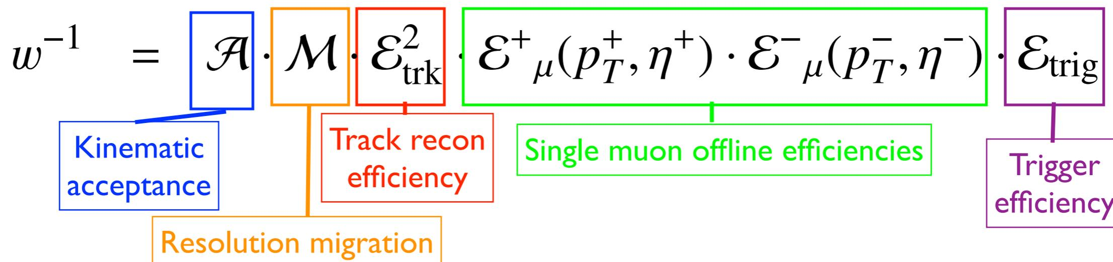
Diagram illustrating the event weighting procedure. The equation is  $w^{-1} = \mathcal{A} \cdot \mathcal{M} \cdot \mathcal{E}_{\text{trk}}^2 \cdot \mathcal{E}_{\mu}^{+}(p_T^{+}, \eta^{+}) \cdot \mathcal{E}_{\mu}^{-}(p_T^{-}, \eta^{-}) \cdot \mathcal{E}_{\text{trig}}$ . The terms are defined as follows:
