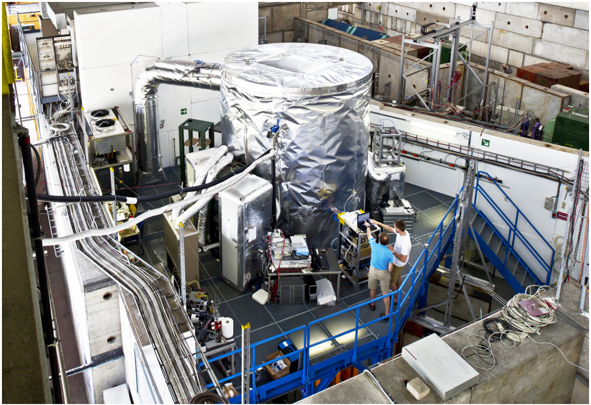
Fig. 1: View of CLOUD in the East Hall T11 zone during the June–July 2010 run. The chamber is surrounded by a thermal housing through which air is circulated via the duct seen to the left. The temperature of the air is controlled to 0.01K stability by a precision thermo-regulator unit seen at the far left. When in operation, the pion beam passes through a counter hodoscope and enters the chamber from the right. The transverse dimensions of the beam at the position of the chamber are around 1.5 \times 1.5 \text{ m}^2 . Instruments surrounding the chamber continuously analyse its contents by extracting small amounts of air through sampling probes.
