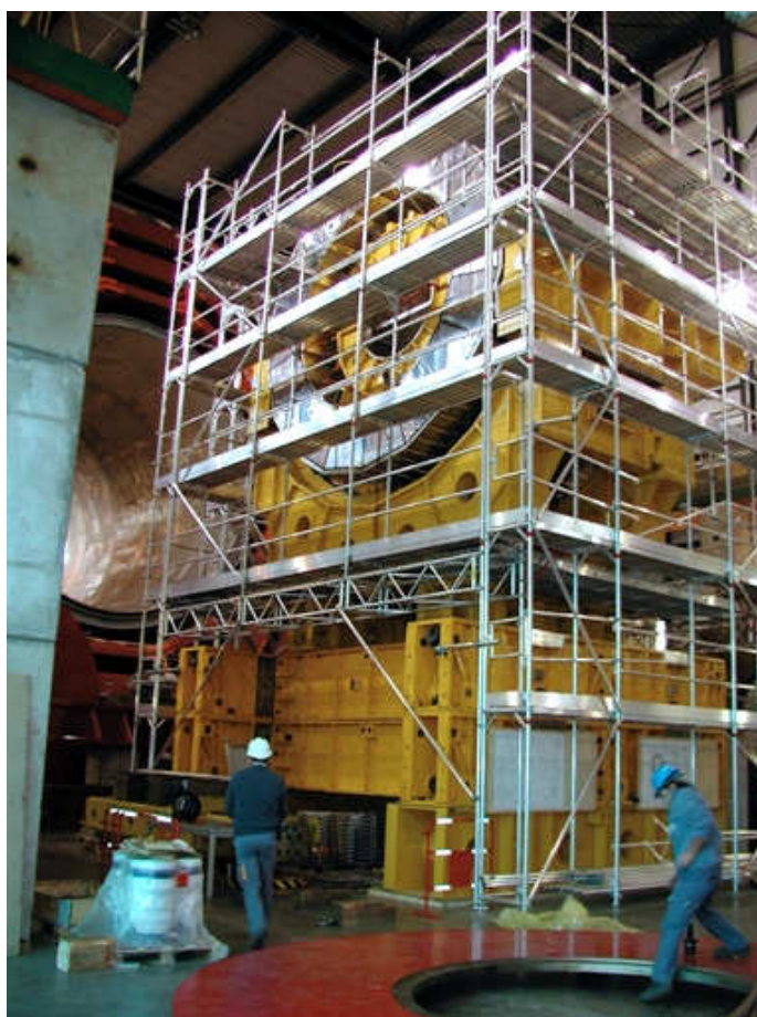
Figure 1.10: An assembled half-barrel of the HCAL.
