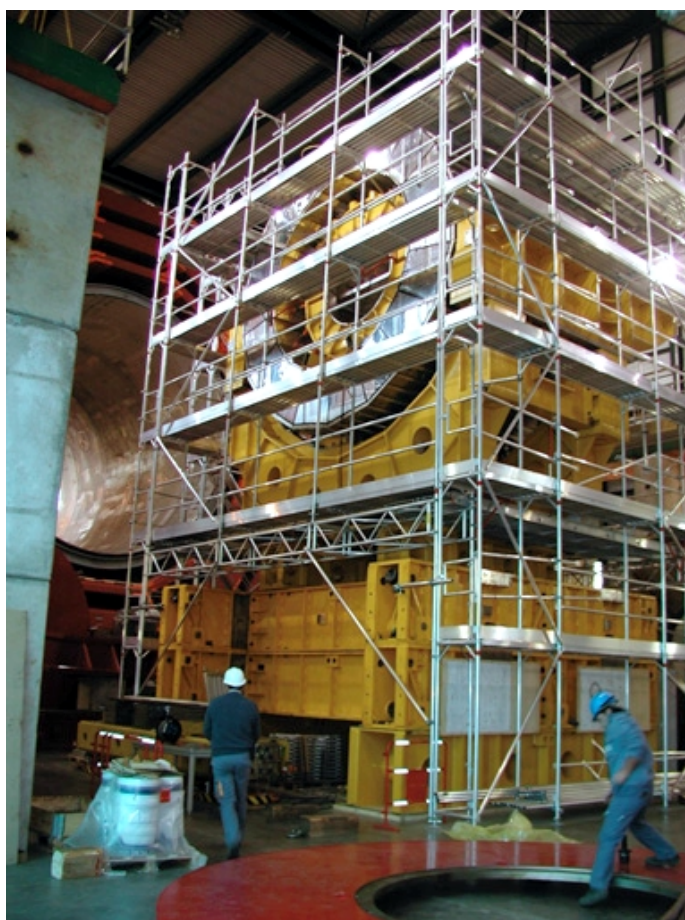
Figure 1.10: An assembled half-barrel of the HCAL.
