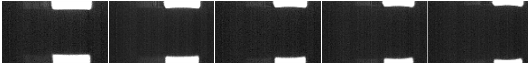
Fig. 7. A sequence of steps of experimental test performed with SHPB filmed with high velocity camera (20.000 fps): due to the friction between specimen and testing equipment the deformation is not uniform (barrelling). The sequence is used to validate the numerical simulations friction model.
