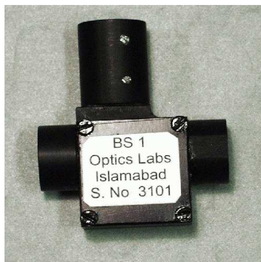
(b) Picture of BS deflection prototype
