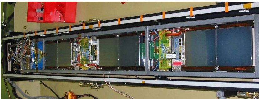
Abbildung A.4.: TOB support structure and front side of a TOB rod with three modules.
