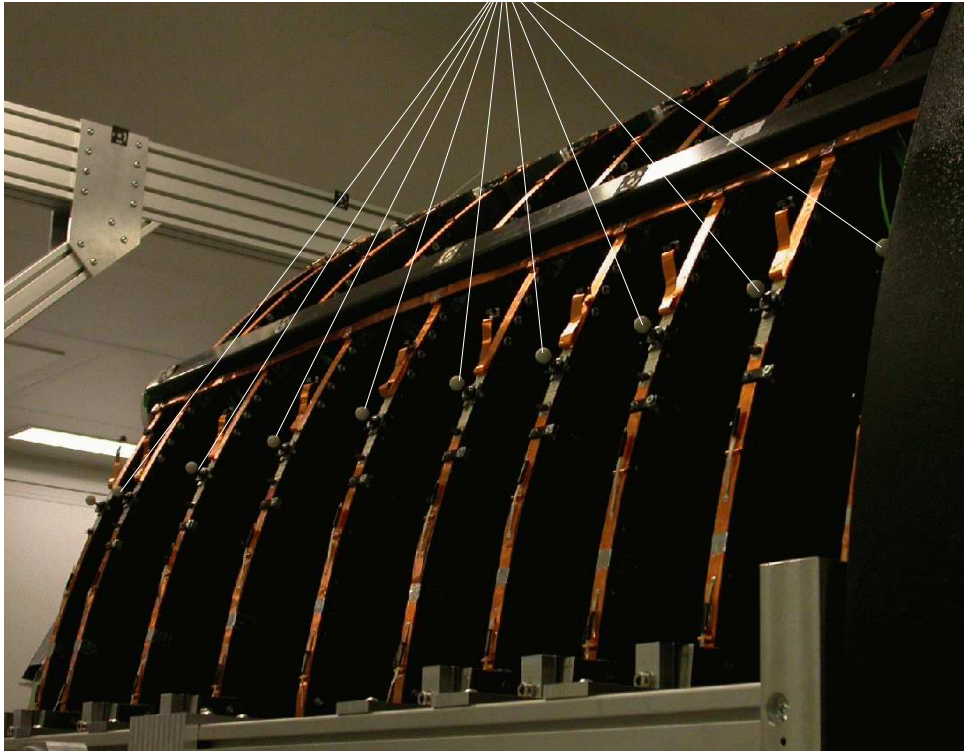
Abbildung I.2.: Spherical survey targets have been fixed on each TEC disc at four positions (figure 5.37). More details can be found in [41].
