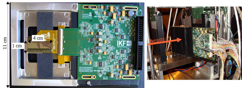
Figure 3: Picture of the first PLUME ladder prototype (left) and its installation on the beam line in November 2009 (right).
