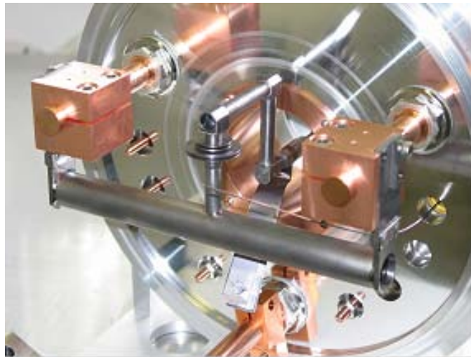
Figure 3.1-7: Quartz transfer line, <warm line> linking to the Ta oven, the ISOLDE target and the ion source.
