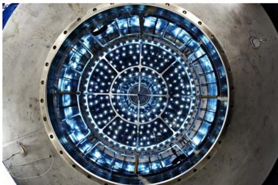
Figure 1. Fisheye image from under the CLOUD chamber: fibre optic illumination and reflections on electropolished interior. (Picture by Maximilien Brice, CERN, Switzerland)
