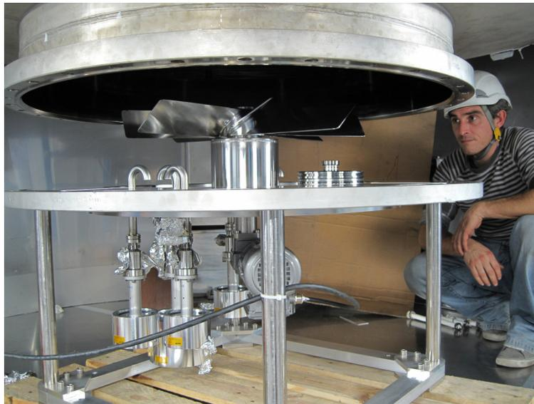
**Fig. 4:** CLOUD internal mixer fan and gas entry valves on the lower manhole cover.
