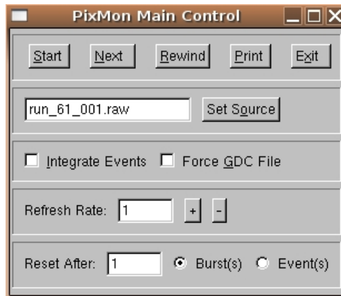
Figure 3.3: Monitoring control panel for the pixel telescope.
