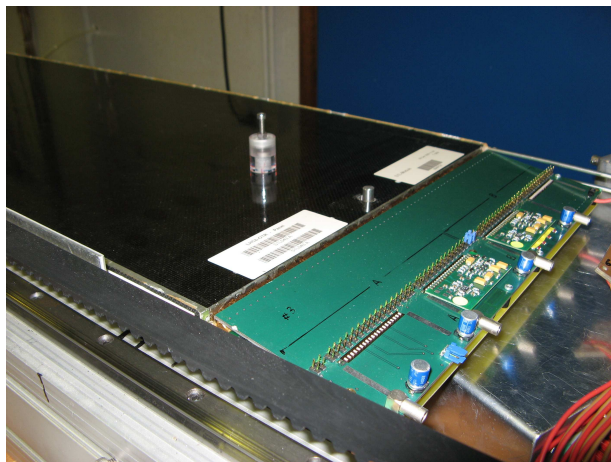
Figure 4.5: Photo of the experimental setup to measure pulse height spectra with an ^{55}\text{Fe} source.
