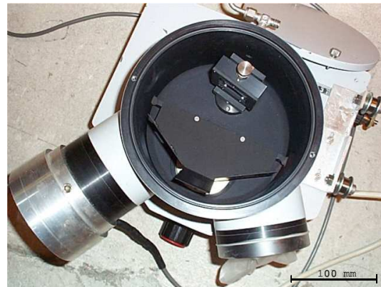
Figure 8.29: Top view photograph into the monochromator.
