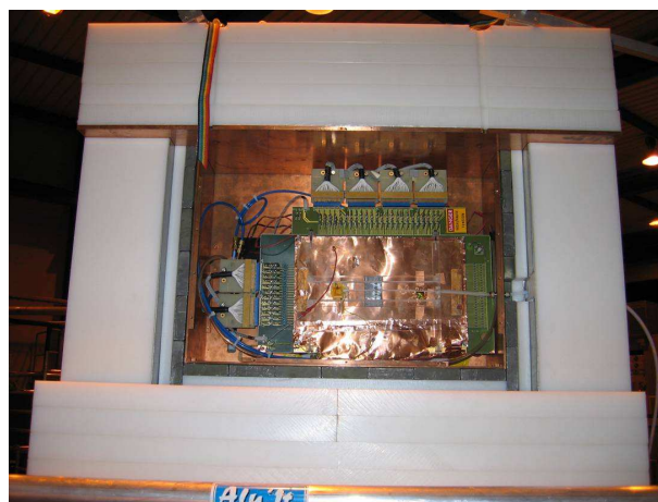
Figure 5.23: Left: Scheme showing the different layers of the TPC shielding. These layers are (from inside to outside): copper (5 mm), lead (2.5 cm), cadmium (1 mm) and polyethylene (22.5 cm). The PVC bag used to enable flushing the complete volume with \text{N}_2 is not included in the picture. Right: Photo of the different layers of the TPC shielding.
