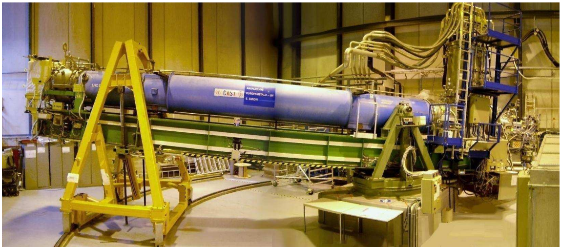
Figure 5.1: Experimental setup of the CERN Axion Solar Telescope. The magnet (blue) is installed on a platform (green), which is supported on the right hand side by a turntable (olive green) allowing horizontal movement. On the other end (left in image), it is carried by two lifting screws at a girder (yellow) for enabling vertical movement. The yellow girder also allows for the horizontal movement along the rails visible on the floor of the experimental hall. Part of the cryogenics plant to cool the superconducting magnet is visible on the right side.
