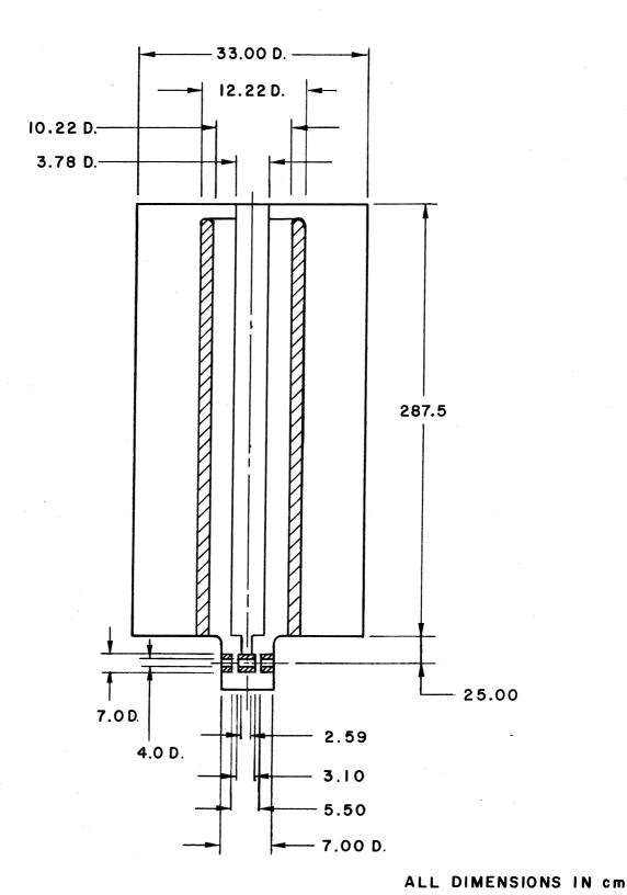
Fig. 3 12.5 MHz Folded Transmission Line Resonator Model with Outside Short
