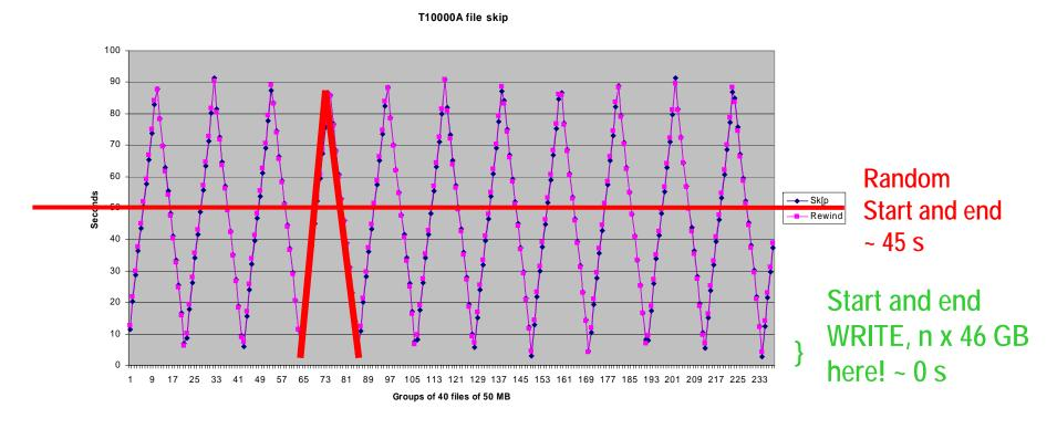
'user' files on tape, each ~50 MB (200 blocks of 256K), simulated labels Here only ~22.5 of 24 track sets are visible, so only 500 of potential 534 GB 'allowed' Command mt -f /dev/nst0 fsf n Command mt -f /dev/nst0 rewind
