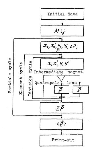
Fig. 2 Block diagram of the program
