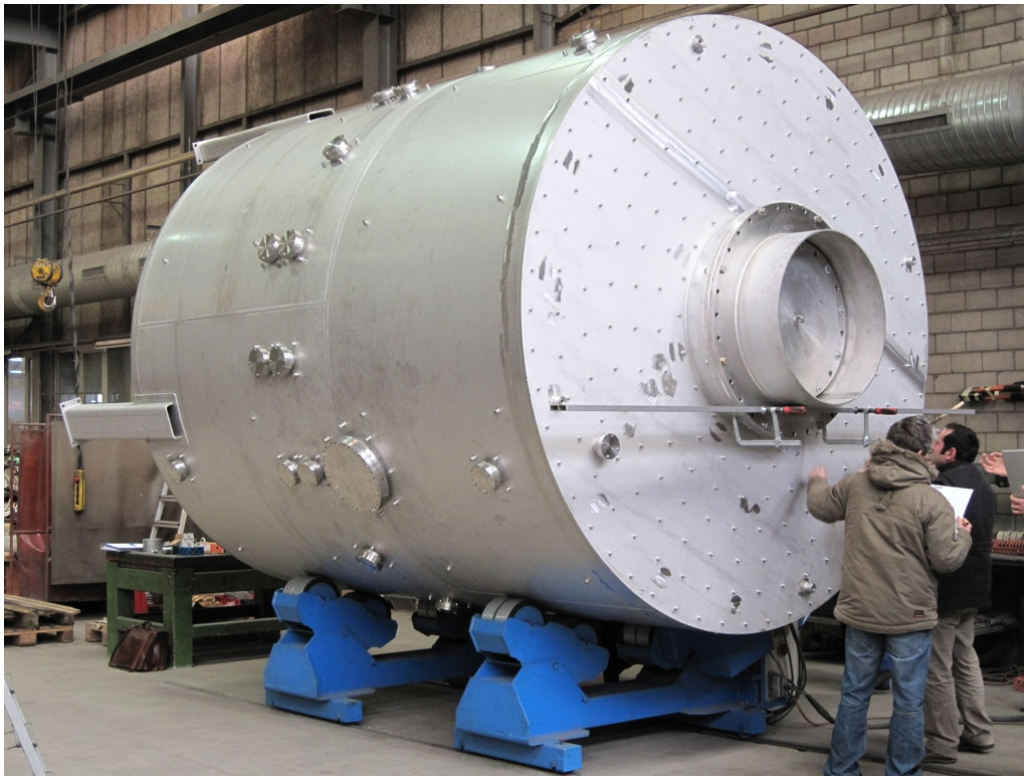
Fig. 12: The 3 m CLOUD-09 chamber under construction at Kasag, Langnau, on 12 March 2009. The UV optical fibre feedthroughs and a 1 m access port can be seen on the top plate of the chamber. The ports on the walls are for sampling probes and optical windows.
