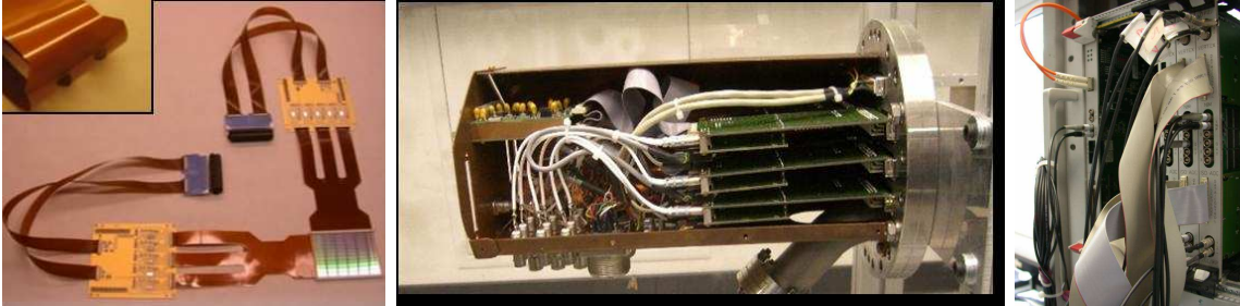
Figure 16: The developed electronic chain: In-vacuum boards with self-triggering chips (left panel), front-end interface boards (center), and complete vertex board with 12 \text{ bit ADC} and sequencer (right panel).
