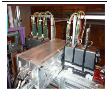
Figure 1: CERN Test beam with Si prototype equipped with SiTR_130-4 chips
