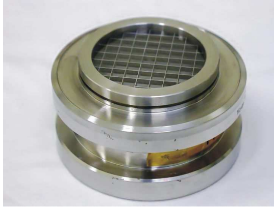
Figure 5.15: View of one of the four cold windows before its installation inside the CAST cryostat.
