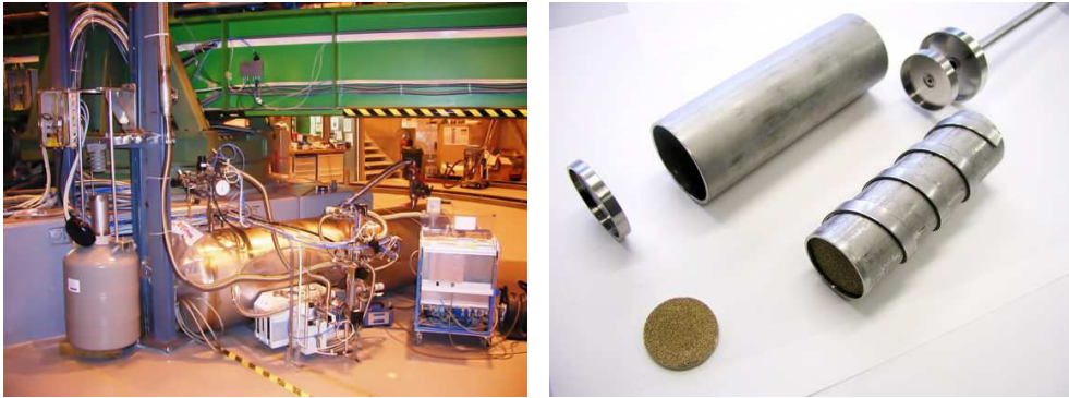
Figure 5.19: On the left the recovery system of the CAST experiment. The right picture corresponds to a detailed picture of the trap used for the gas purification.
