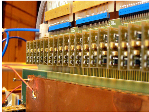
Figure 6.4: Array of 24 ALCATEL SMB302 4-channel preamplifier chips used for the cathode signals of the TPC.
