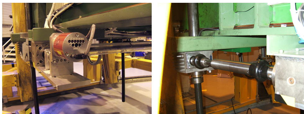
Figure 5.7: Image of the Vertical movement system of the CAST magnet (left) and its encoder (right).
