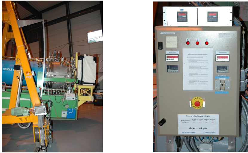
Figure 5.8: Image of the Horizontal movement of the CAST magnet (left) and the encoder readers for both, vertical and horizontal movement (right).
