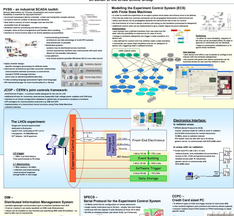
• DIM server running on CCPC or SPECS master PC publishes services to DIM Nam Server (DNS) from where the client (ECS) can subscribe to it. Data exchange peer to peer from server to client
